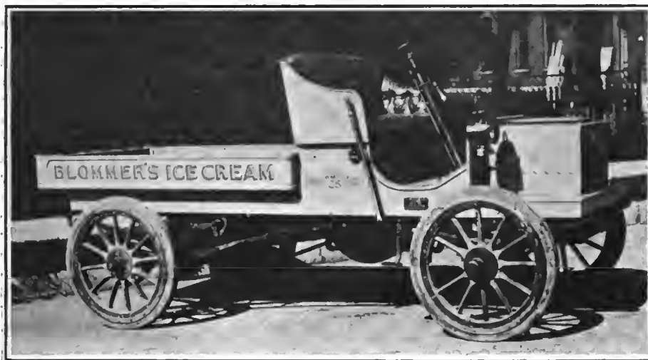
CLEMICK-HIRSCH TWO-TON, OPEN-BODY DELIVERY WAGON, WITH 24-HORSEPOWER DOUBLE-OPPOSED CYLINDER ENGINE.
